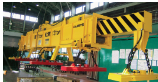
(Lifting steel plates)
